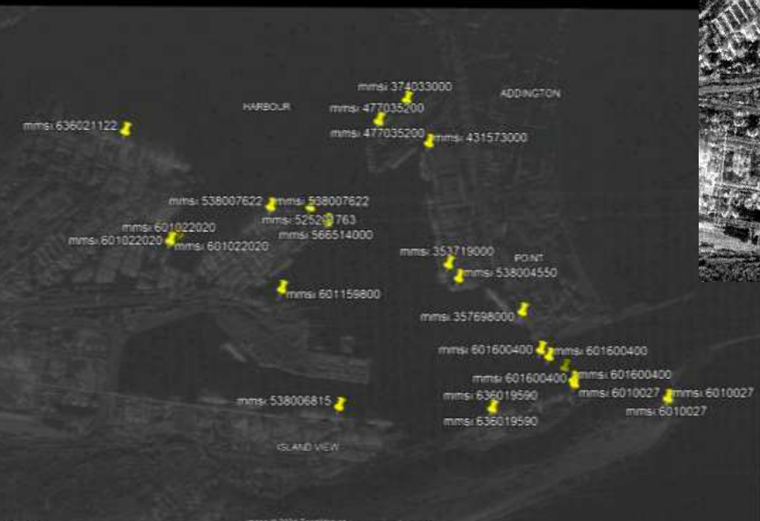
Geo-located SAR Image as displayed in Google Earth showing AIS logs (Note colour of SAR image not displayed properly in Google Earth)
